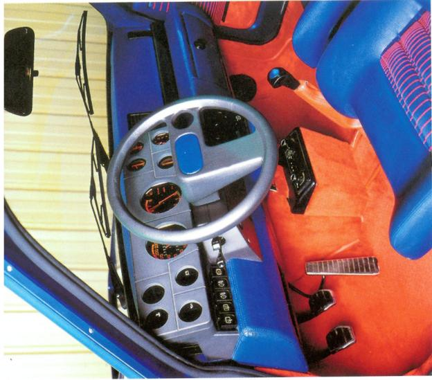
a vertical median line. The Instruments and switches were permanently back lit with a gentle red glow whenever the ignition was switched on, these can be controlled by a variable rheostat control switch. The steering wheel was striking in appearance and almost "Art Deco" in design, being a two spoke L shaped wheel with a coloured centre. A Toolbox was mounted on the engine cover containing a fine set of Facom tools and a pair of Kid leather gloves.
