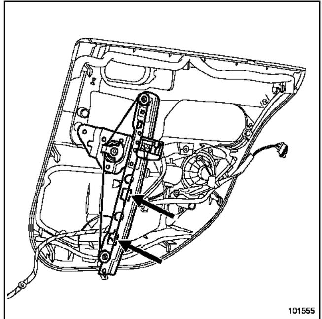
Clip the motor assembly on the lining.
