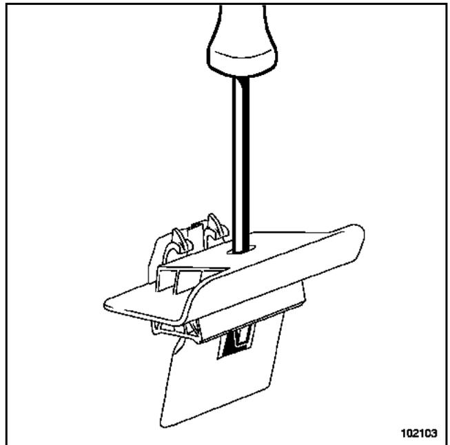
Pressing down the screwdriver, release the clip.
