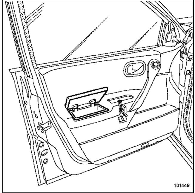
Unclip the glove compartment from the door.
