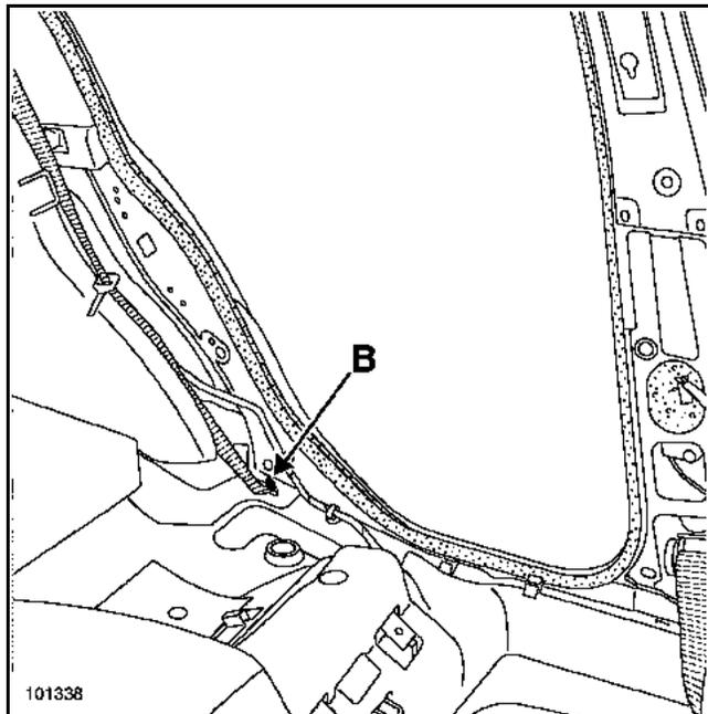
Remove the seat belt lower mounting bolt (B).
