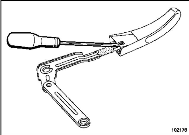
Unclip the seat booster cushion handle using a flat screwdriver.
