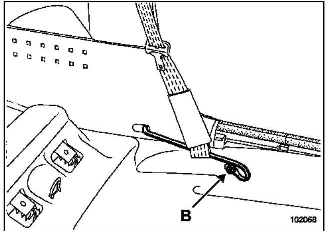
Remove the seat belt rail bolt (B).
