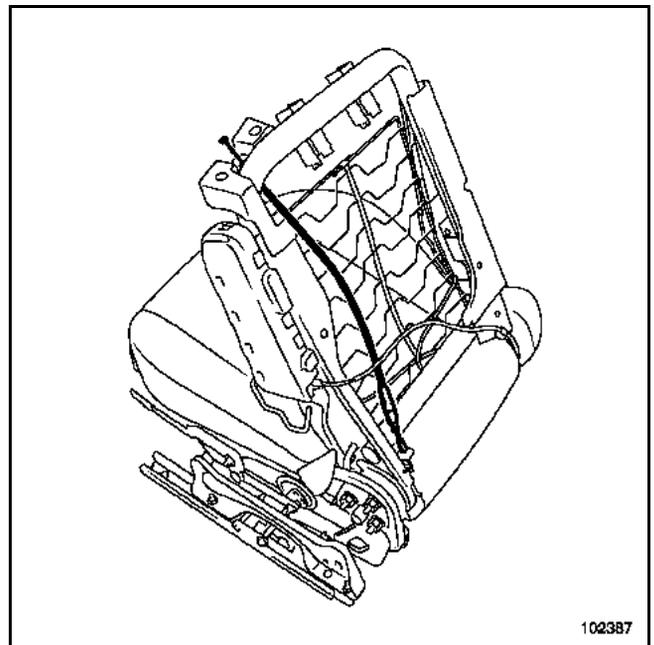
Unclip the cable stops.
