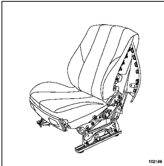
Unclip the cover clips at the airbag.
