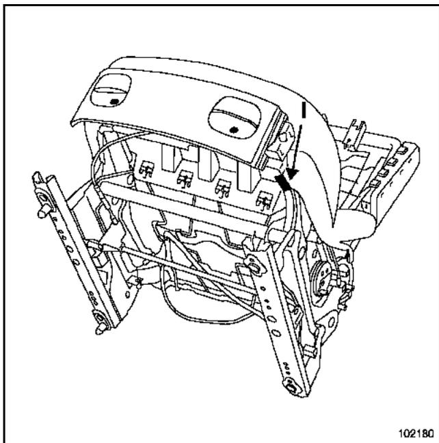
Release the cover retaining section (I).
