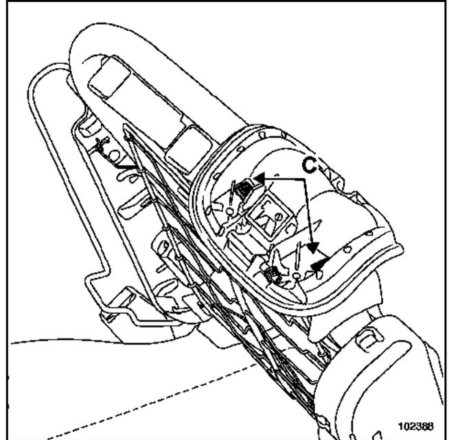
Release the seatback unlocking mechanism cable thrust bearing.
