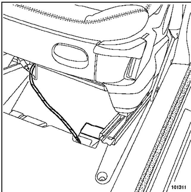
Disconnect the connector under the seat.
