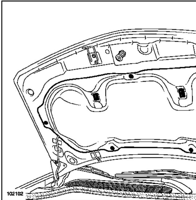
Unclip the clips (five clips) using an unclipping tool.
