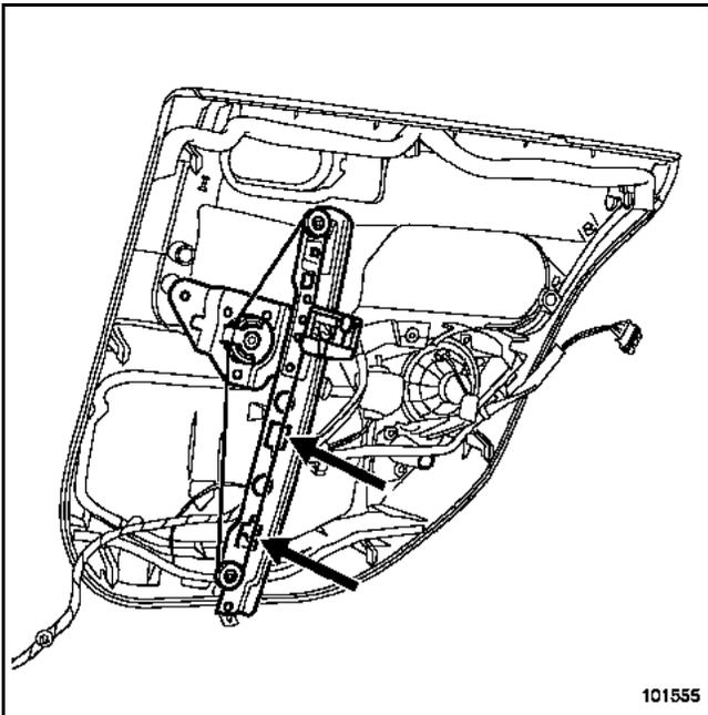
Disconnect the window riser motor.
