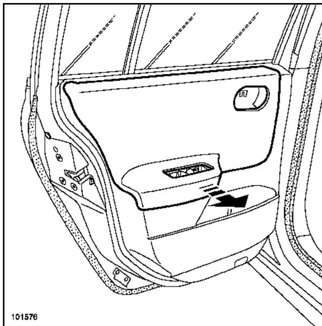
Unclip the lining flap with an unclipping tool (while protecting the lining).
