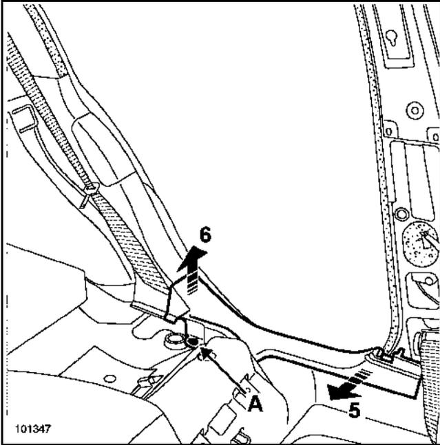
Remove clip (A) using unclipping pliers.
