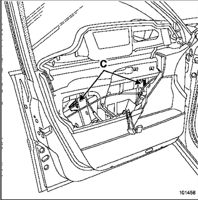
Position the window in order to access the two mounting clips (C).
