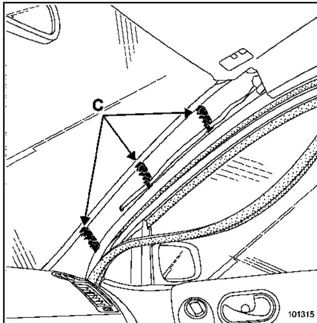
Before refitting the trim, check the condition of clips (C), Part no.: **82 00 100 314**.
