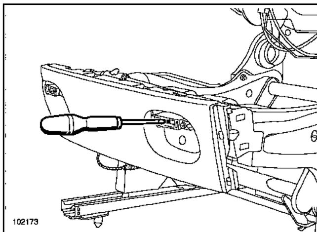
Detach the unlocking control cables.
