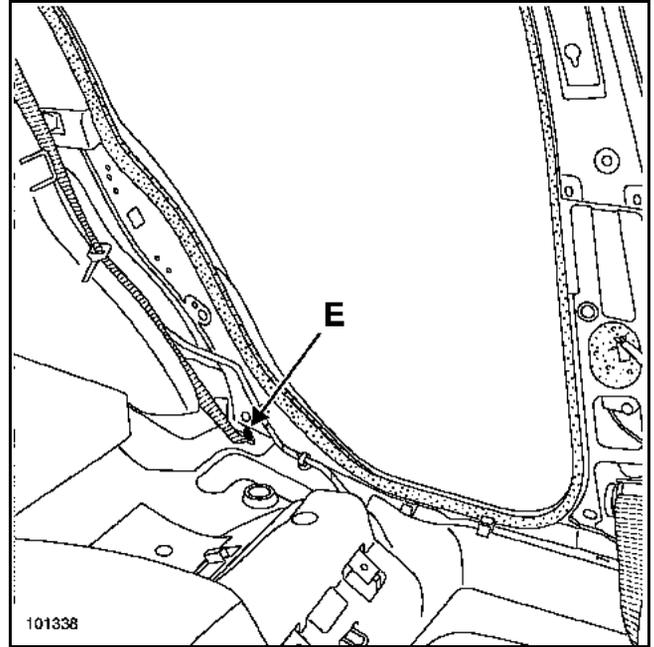
Remove the seat belt lower mounting bolt (E).
