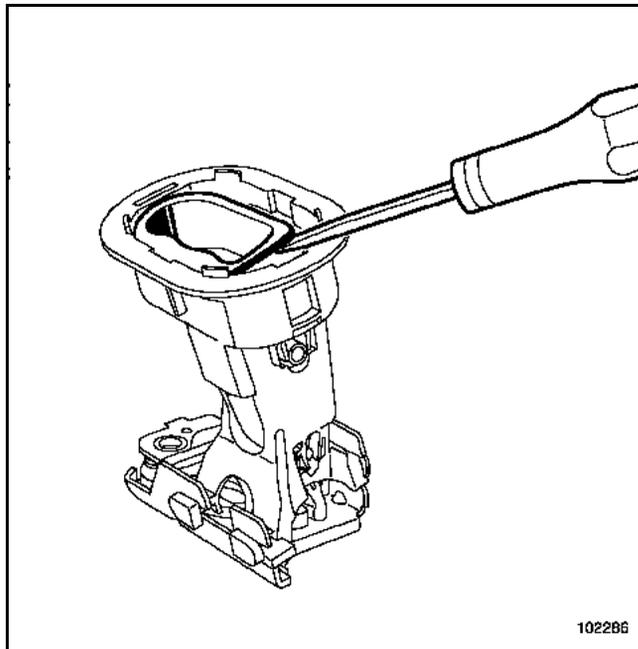
Unclip the seatback unlocking control.
