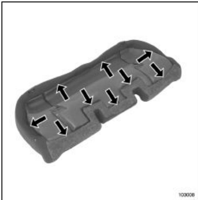
Remove the cover retaining sections.
