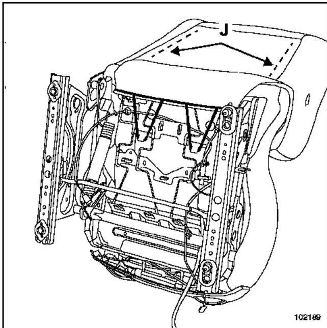
Release the lower retaining rubber bands from the seatback cover.
