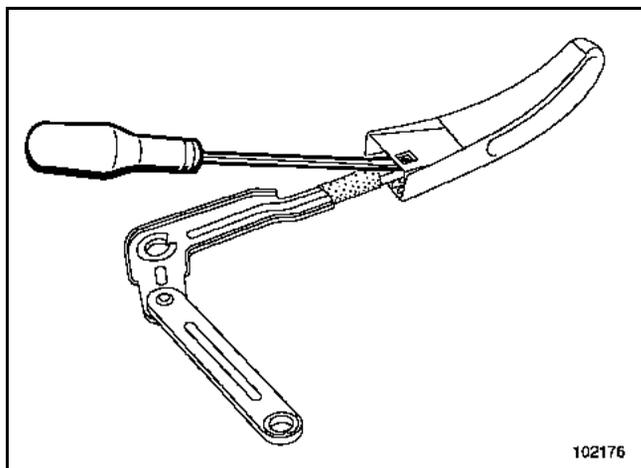
Unclip the seat booster cushion handle using a flat screwdriver.
