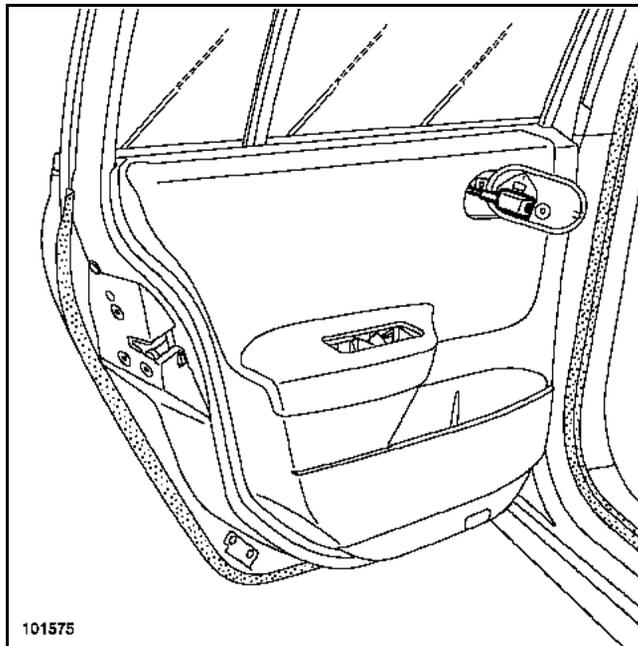
Using a flat screwdriver, unclip the opening release cable mounting cover.
