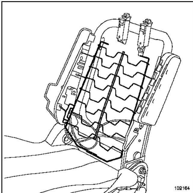
Remove the fabric from the lumbar adjustment mechanism.
