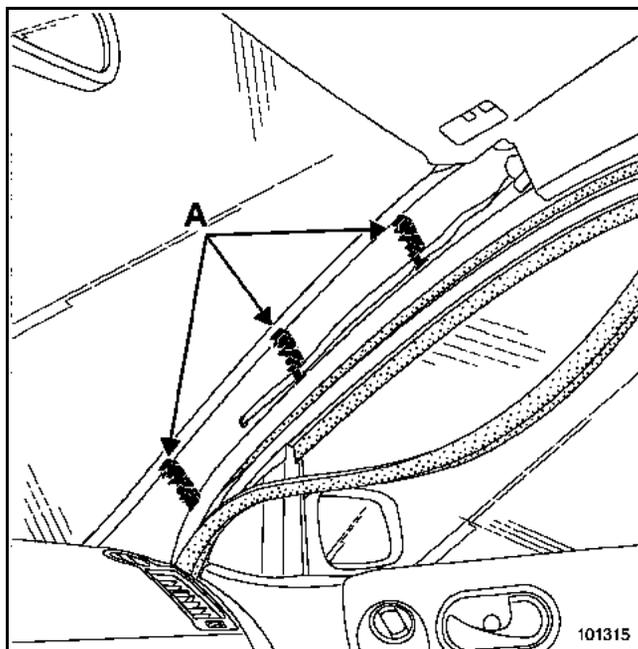
Before refitting the trim, check the condition of the clips (A), Part no.: **82 00 100 314**.
