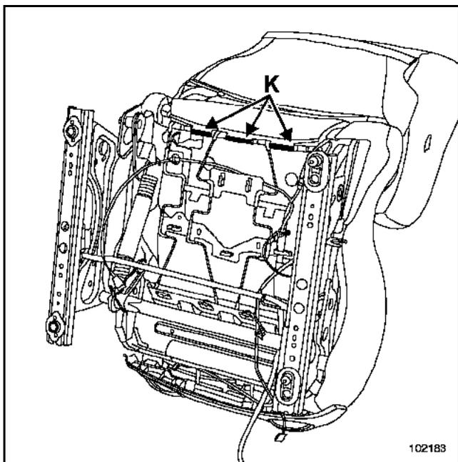
Remove the cover retainer profiles (K).
