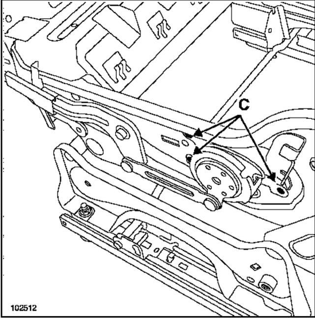
Remove the seat booster cushion adjustment mechanism rivets (C).
