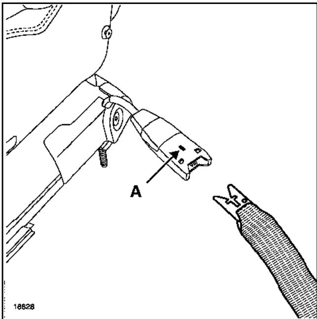
Unhook the seat belt by pressing on latch (A).
