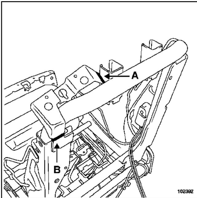
Cut the seatback unlocking mechanism plate along marks (A) and (B).
