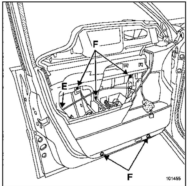
Disconnect the lock connector (E) and the two handle module connectors (if the vehicle is equipped with the hands-free function).
