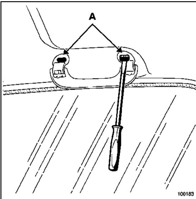
Using tool **Car. 1597**, unclip the two mounting pins (A), then pull it to remove.
