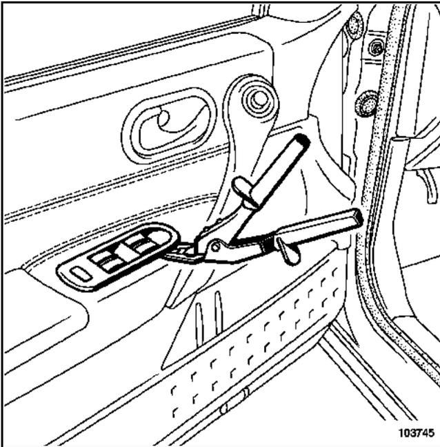
Protect the lining (e.g. with a mastic knife), and unclip the electric window plate using the unclipping tool.
