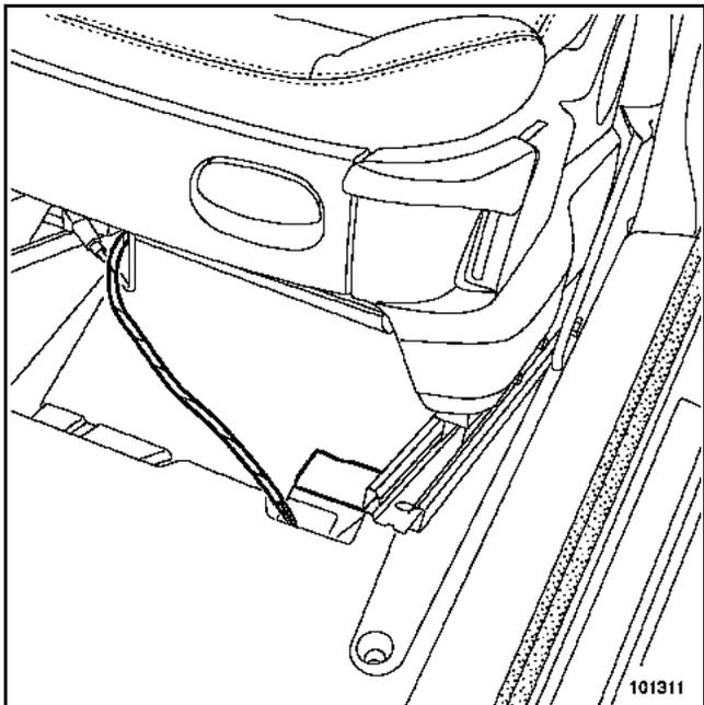
Disconnect the connector under the seat.
