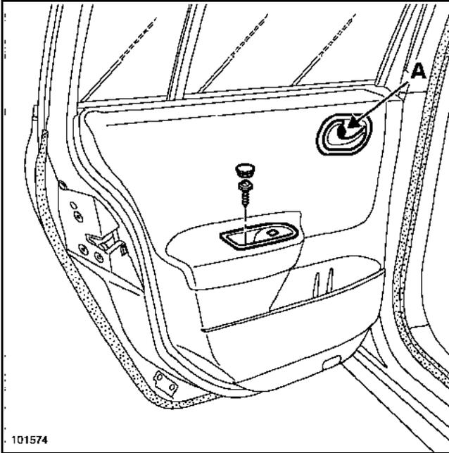
Remove the window lift plate cover and bolt.
