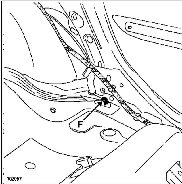
Remove the seat belt lower mounting (F).
