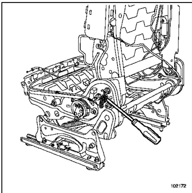
Unclip the seatback unlocking tie-rod.
