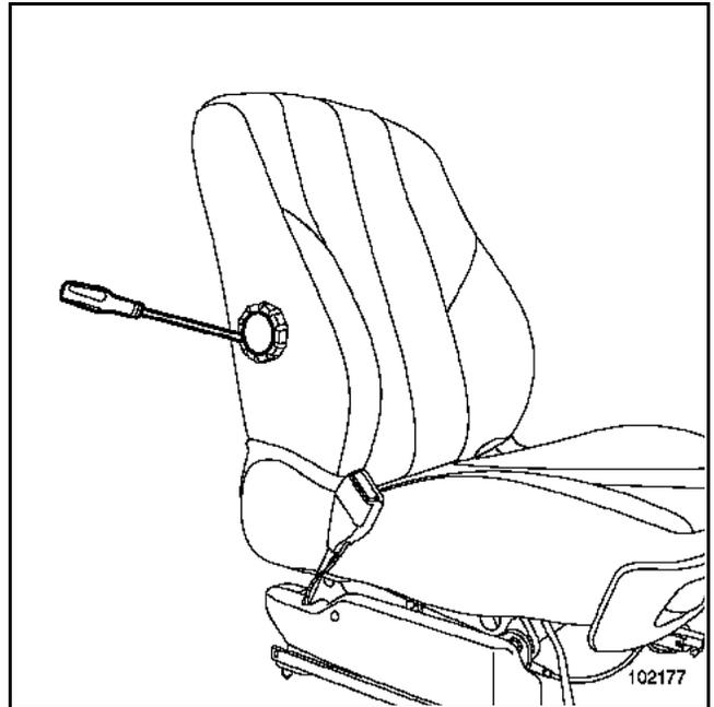
Remove the lumbar support adjustment tumblewheel mounting cover, using tool **Car. 1597**.
