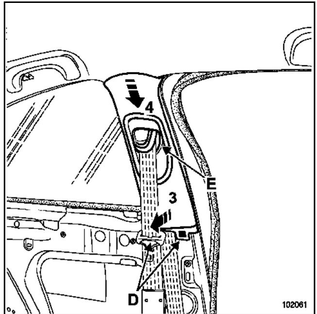
Partially remove the door seal.
