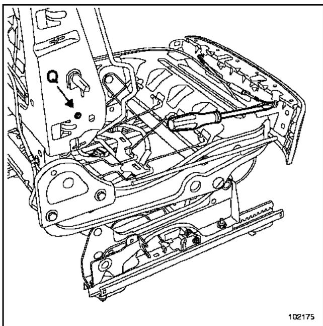
Remove the control cable sheath stops.
