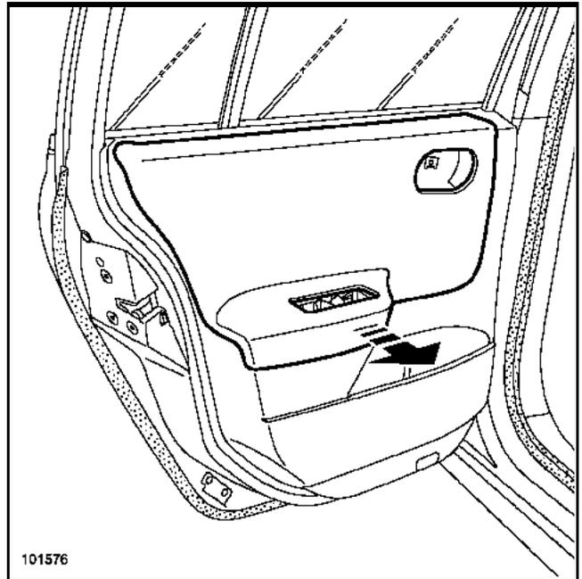
Unclip the trim flap using an unclipping tool (while protecting the lining).
