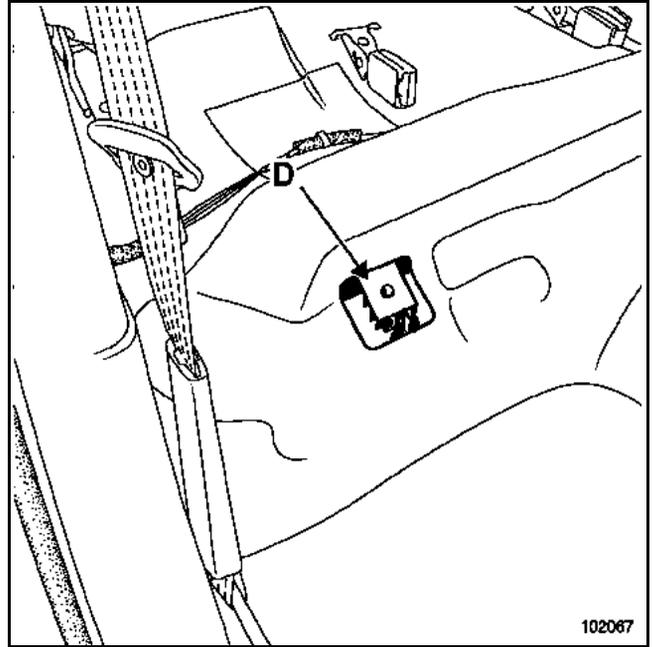
Insert a screwdriver into opening (D).
