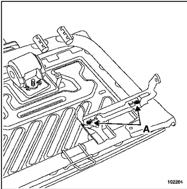
Remove the arm rest mounting bolts (A).
