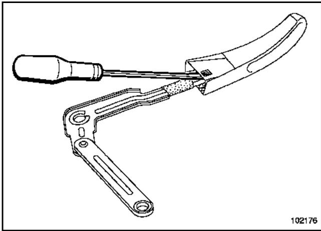
Unclip the booster cushion handle using a flat screwdriver.
