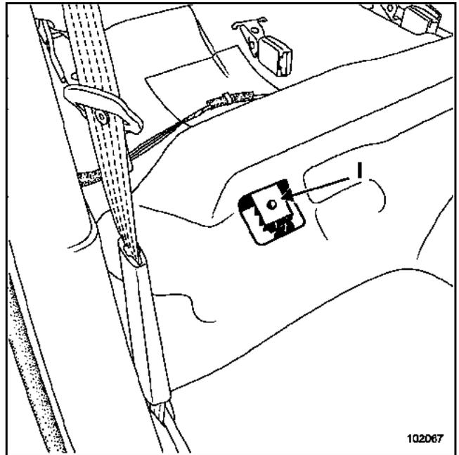
Insert a screwdriver into opening (I).
