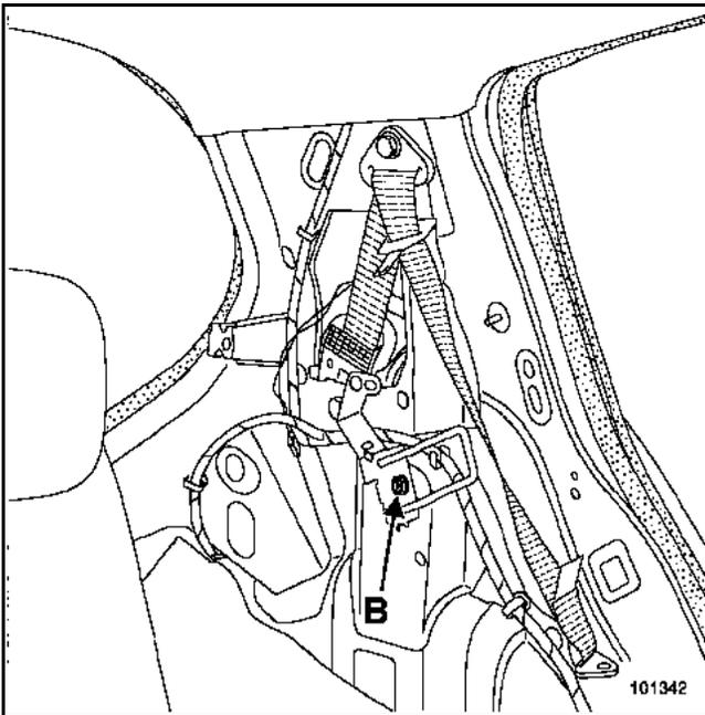
Remove the seatback striker mounting bolt (B).
