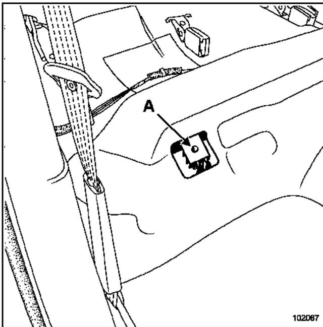
Insert a flat screwdriver into hole (A).
