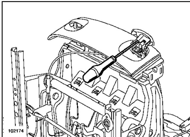
Remove the runner adjustment handle fastening bolt.
