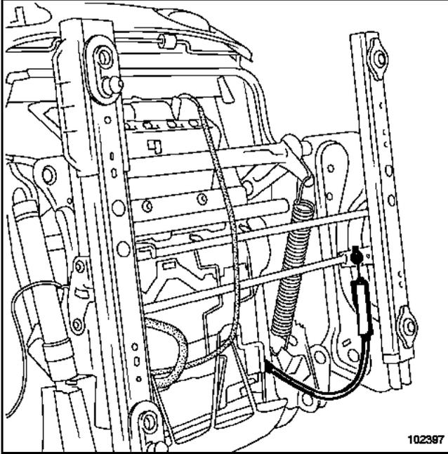
Unclip the cable stop to free the seatback unlocking control.
