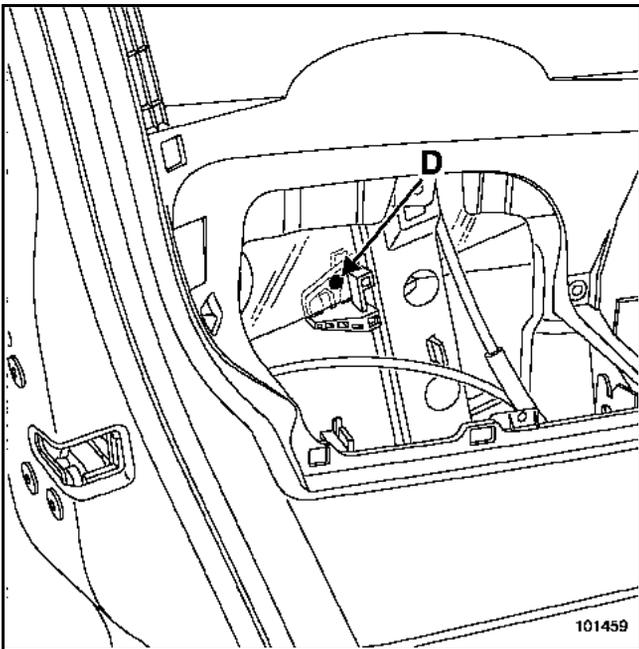
Release the catch (D) by pulling the window upwards.
