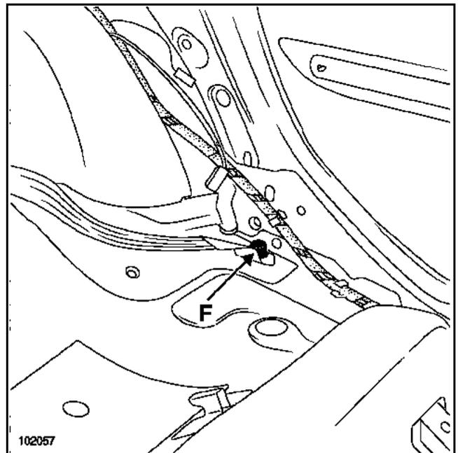
Remove the seat belt lower mounting (F).
