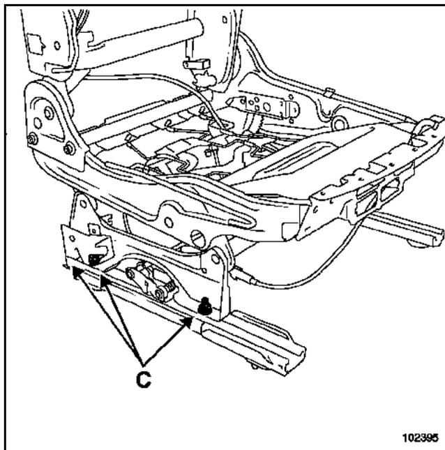
Remove the three nuts (C).
