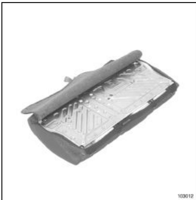
Partially remove the lining to access the headrest guides.
