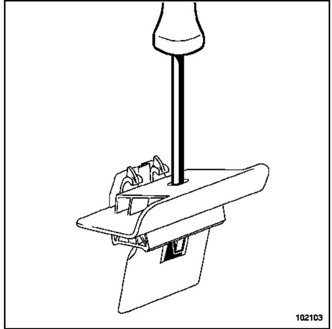
Pressing down the screwdriver, release the clip.
