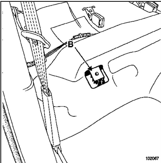
Insert a screwdriver into opening (B).
