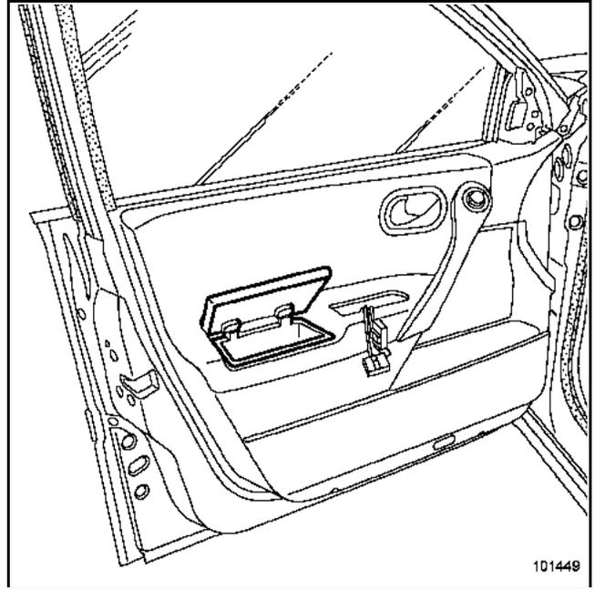
Remove the glove compartment from the door.
