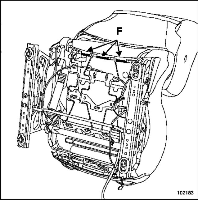
Remove the seatback cover retaining sections (F).
