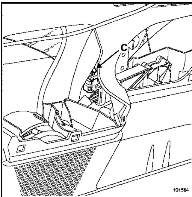
Remove the catch (C) by pulling the window upwards with a flat screwdriver.
