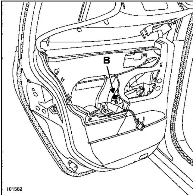
Position the window in order to access the two mounting clips (B).
