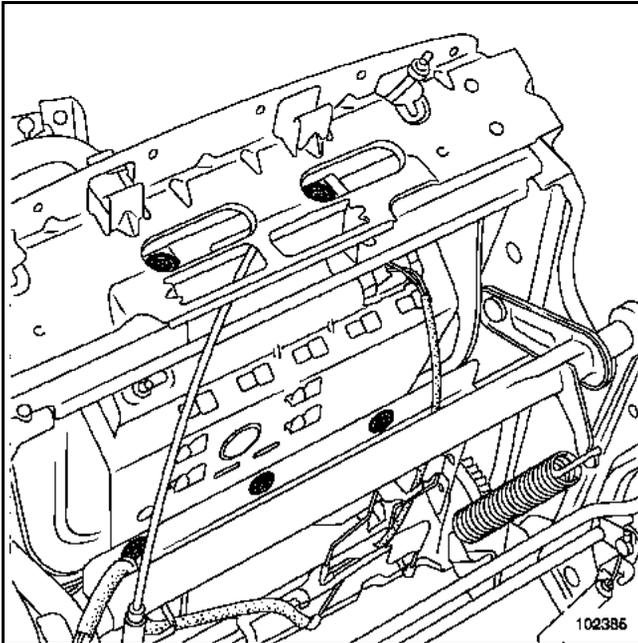
Remove the anti-submerging airbag mounting bolts.
