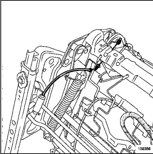
Unclip the cable stops.
