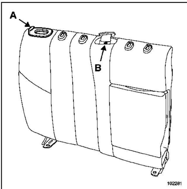
Unclip the unlocking mechanism trim (A).
