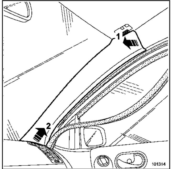
Partially remove the seal.
