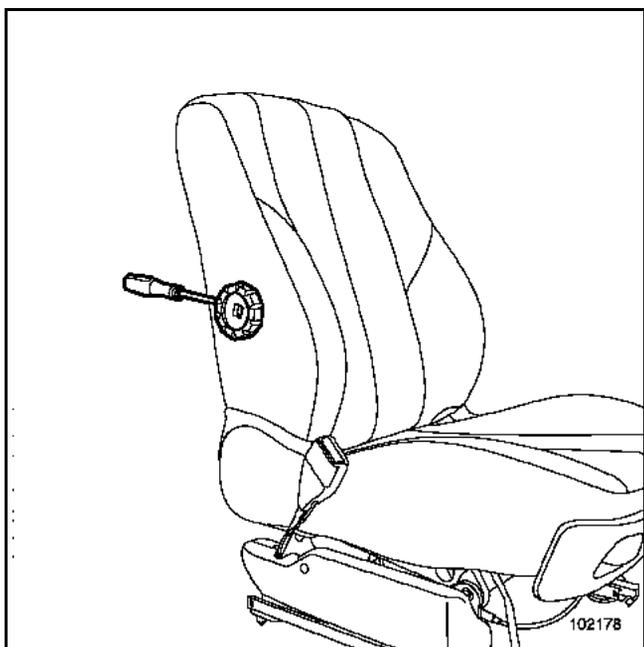
Using a screwdriver, remove the lumbar support adjustment tumblewheel.
