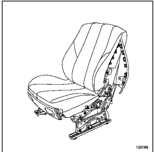
Unclip the cover clips at the airbag.
