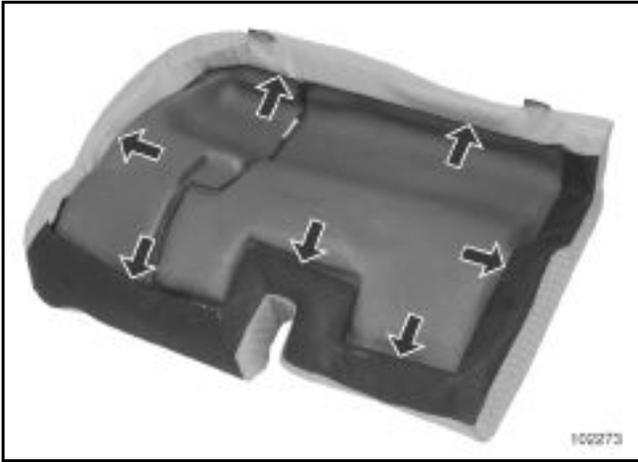
Remove the cover retaining sections.
