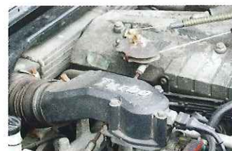
Check all the intake and boost hoses for splits.
